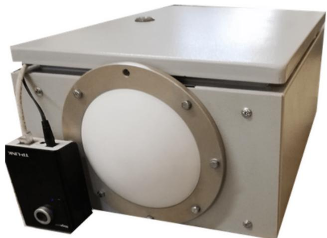
76 GHz band for this radar has been chosen because of sharp recognition any objects that are large than its wavelength of 4 mm.
