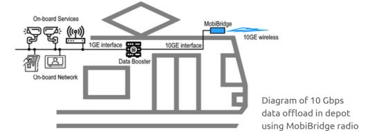
MobiBridge 10G is the industry's first 10 Gbps per channel radio designed to download and upload video, data and other content at railway stations and depots, at metro stations, as well as on high-speed tram stops and along the routes.
