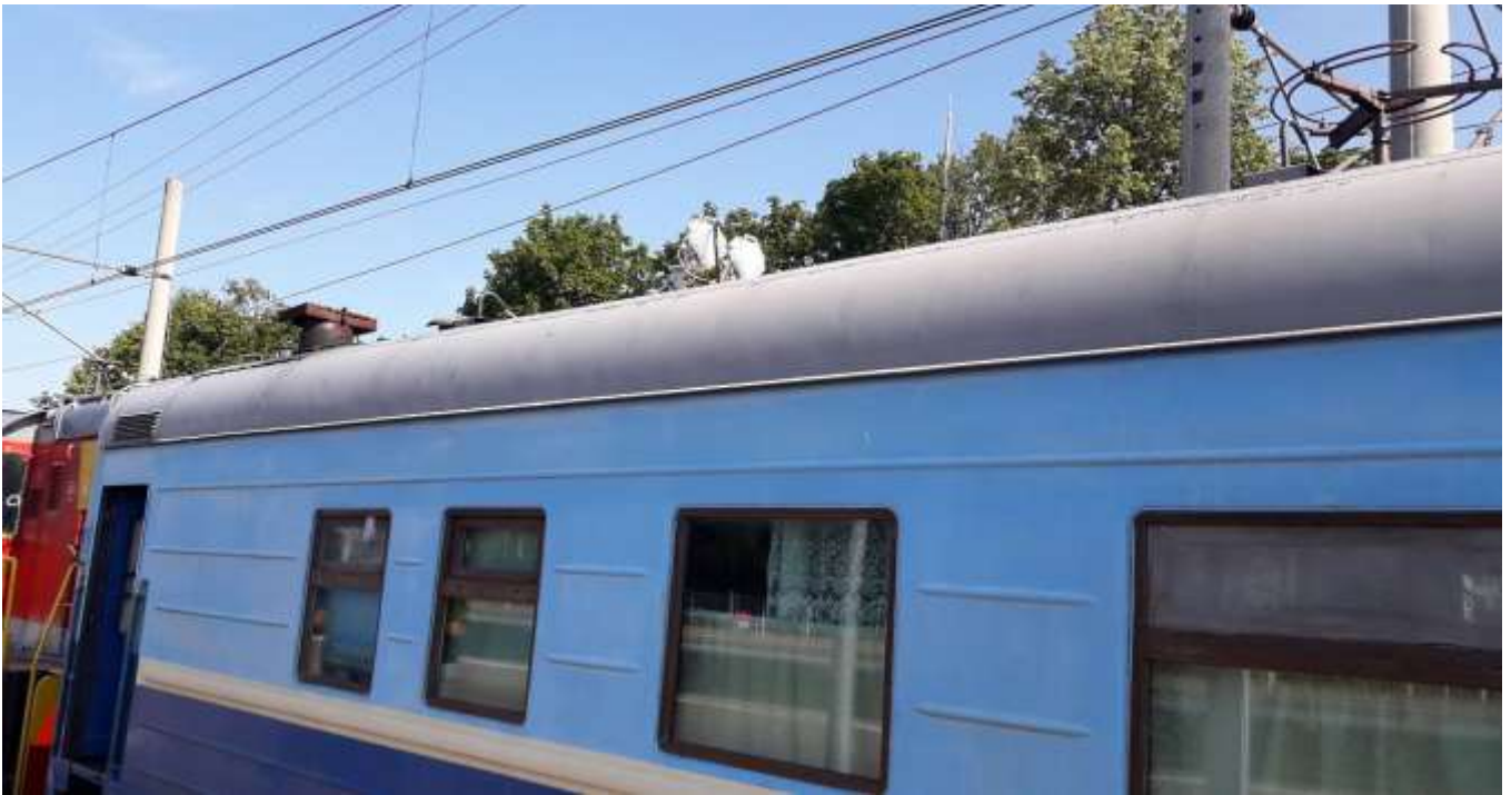
Photo of the PPC-10G-Rail radios on the roof of the lab carriage
