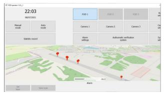
The FOD operator software displays target marks on the electronic map of the airfield. A log is generated with a description of the target, including detection time, signal levels, and GPS coordinates. The radar provides target coordinates for the PTZ HD Multispectral Camera system. The specifications of the electronic optical video monitoring system are configured for a specific runway. An integrated control system remotely monitors radar serviceability 24/7.
