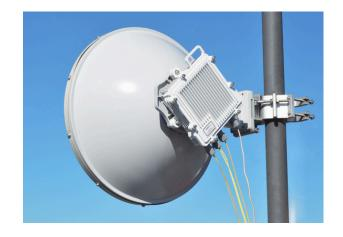
Radios in both E-band and Q-band are shipped with 1 ft or 2 ft antennas, and 3 ft antennas are also available for Q-band radios to allow industry-record distance range.
