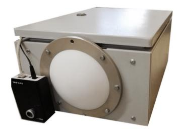
76 GHz band for this radar has been chosen because of sharp recognition any objects that are large than its wavelength of 4 mm.
