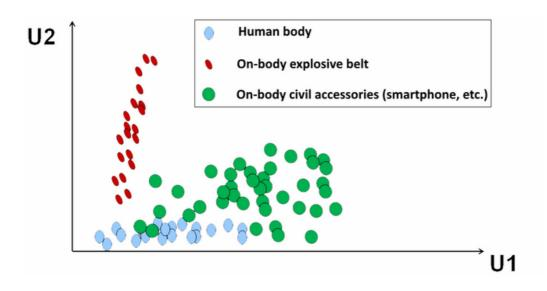
Analysis of typical reflected signals has allowed ELVA's researchers to identify patterns that are reflected from ordinary objects on the human body and hidden weapons.
