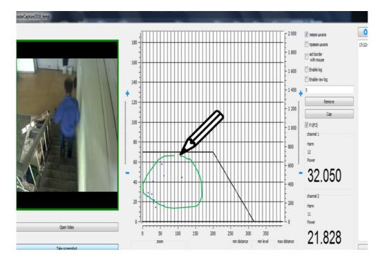
A person who has no hidden metal particles, so the threshold is not exceeded, the green light is ON.
