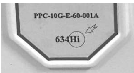
Fig. 32. Example of PPC-10G label with Hi symbols on the back of the radio body
