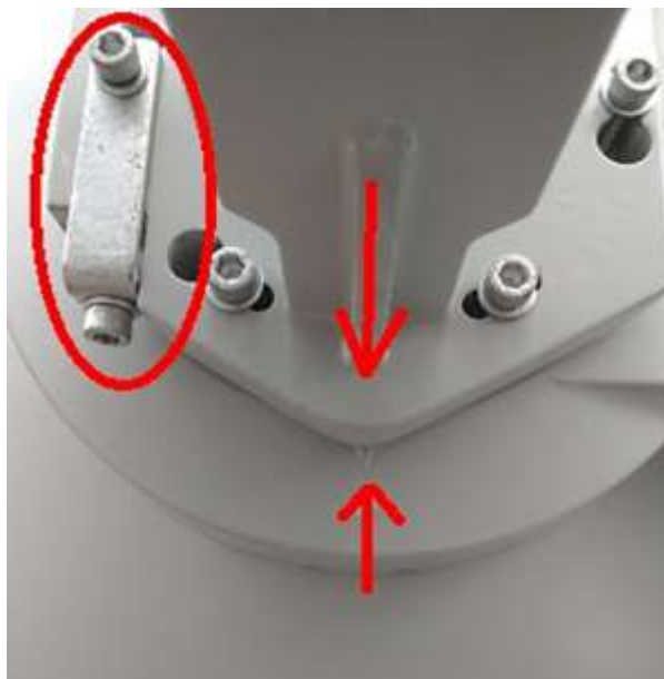
Fig. 47. Adjust the diplexer rotation using the element marked by red oval
