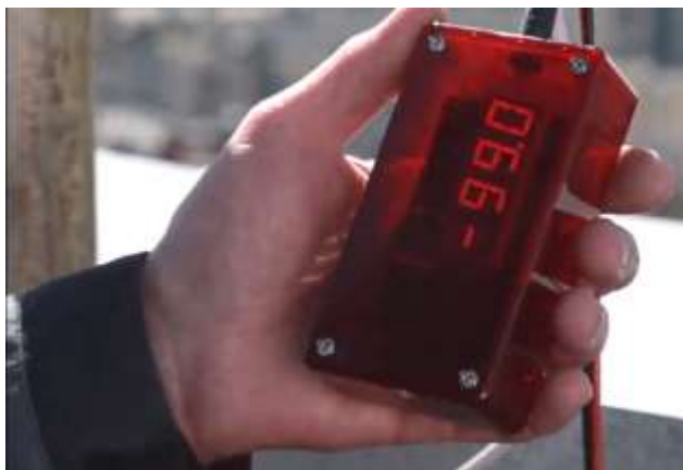
Fig. 28. During antenna alignment, RSL indication should change from -99 to actual "RSL at alignment mode" value for your distance according Link Budget Calculator (see http://linkbudgetcalc.elva-1.com )
