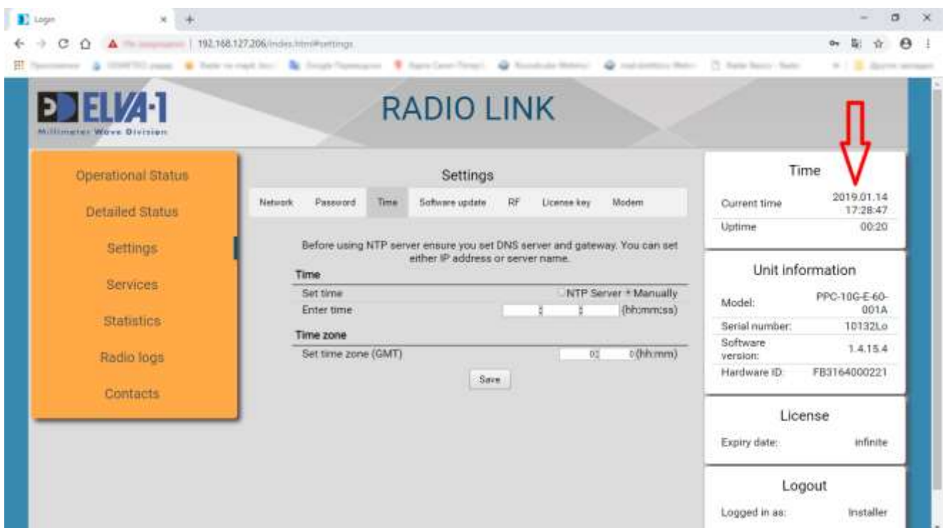
Fig. 38. Check and if necessary adjust actual time settings for the radio
