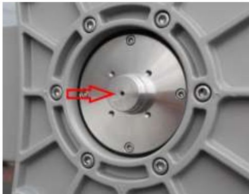
Fig. 18.. Remove protective tape waveguide hole on antenna and transceiver
