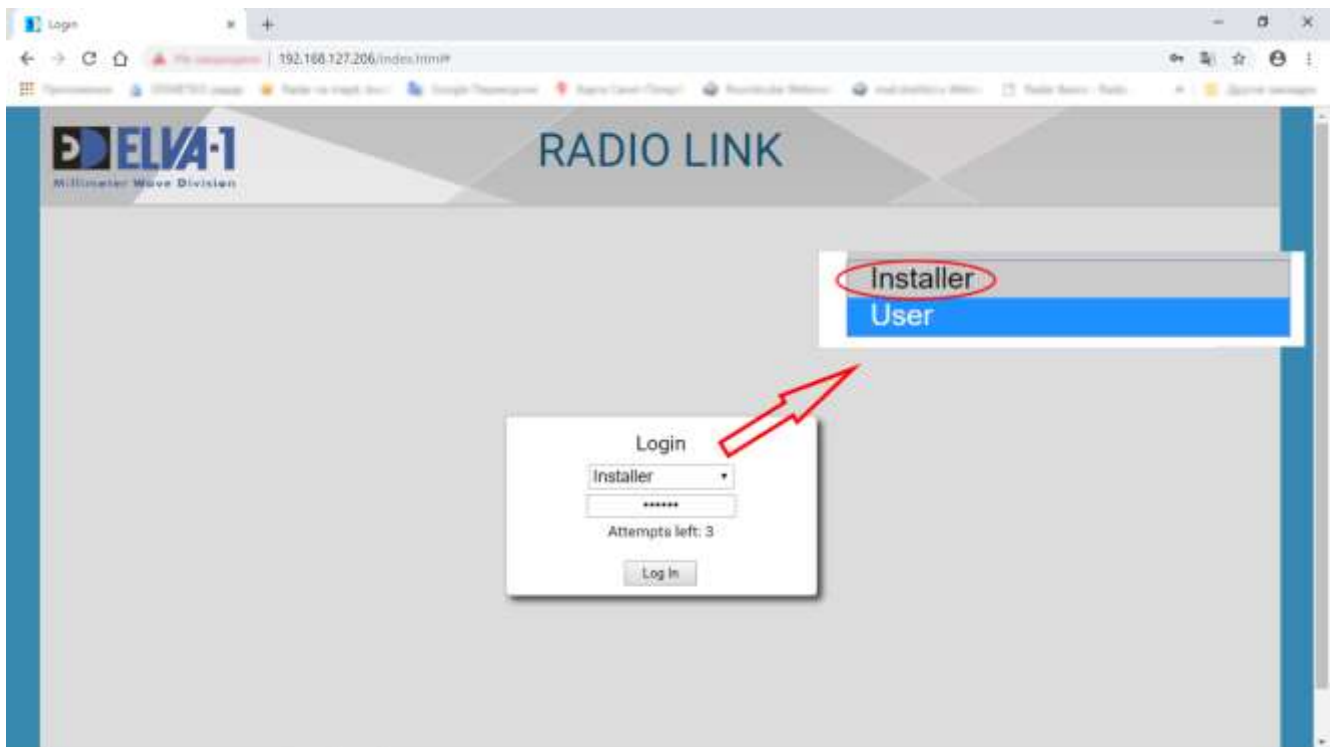
Fig. 35. Login as Installer with default password 111111
