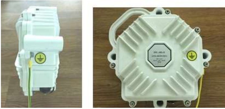
Fig. 22. Grounding wire position
