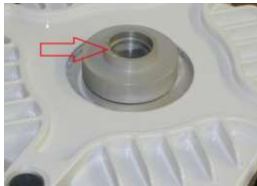
Fig. 18.. Remove protective tape waveguide hole on antenna and transceiver
