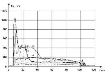
During summer 2002 time, our engineers visited customer sit radiometer tuning and a series of plasma experiments. These measurements at 52GHz to 75GHz on second harmonic of ele frequency. ELVA's ECE Radiometer was used to register an experiment content emission at a mode of plasma heating by *I* measured dependence of electron temperature vs time for va shown in Fig.2.
