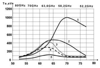
plane. The measured dependence of electron temperature  $T_e$  vs torus radius R for various points of time is shown in Fig.3.
