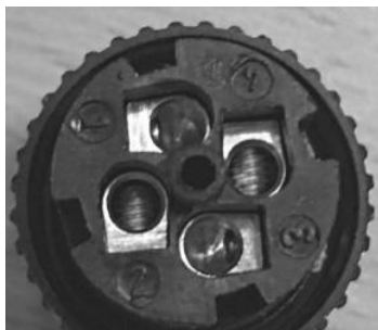
Fig. 13. DC power connector pins
