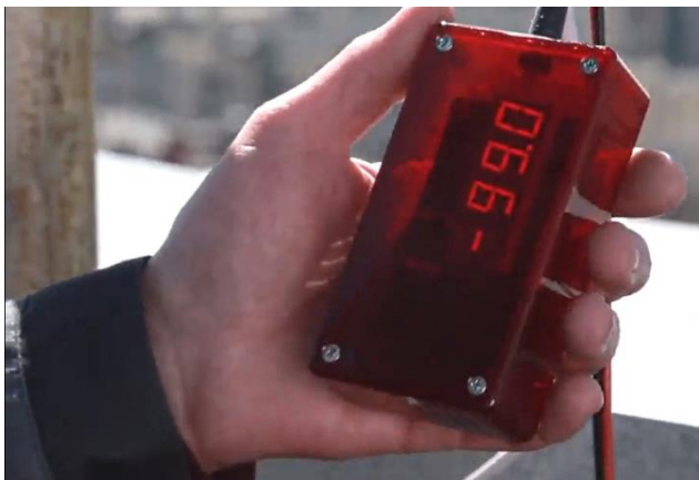
Fig. 28. During antenna alignment, RSL indication should change from -99 to actual "RSL value" for your distance
