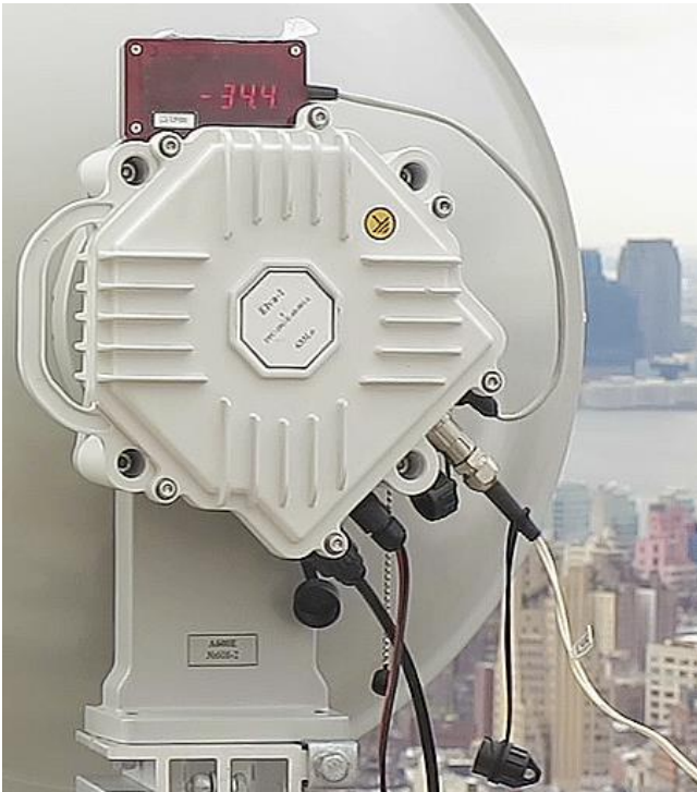
Fig. 30. Do not forget to remove RSL meter and close its socket on the transceiver with ribbon cap when antenna alignment will be complete
