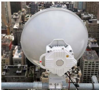
Fig. 9. Radio could be installed on vertical or horizontal pipe
