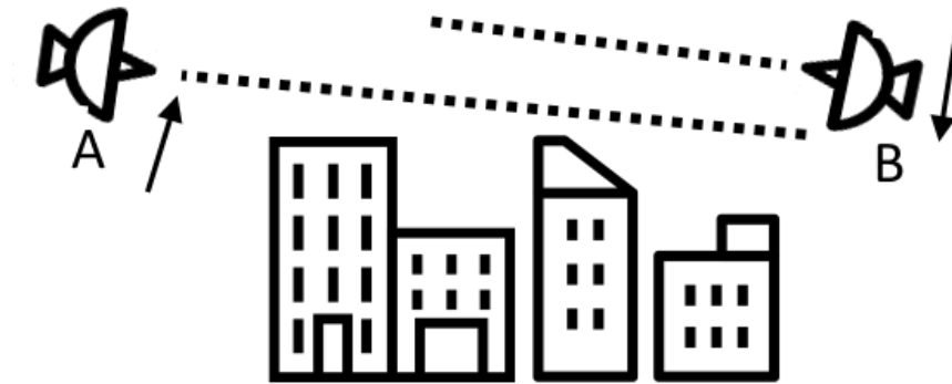
Fig. 26. Antennas A and B to an alignment that is above (B) and below (A) the LOS.
