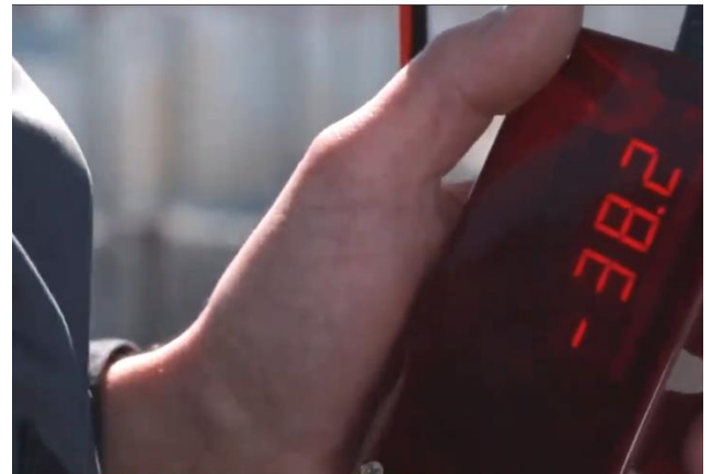
Fig. 28. During antenna alignment, RSL indication should change from -99 to actual "RSL value" for your distance
