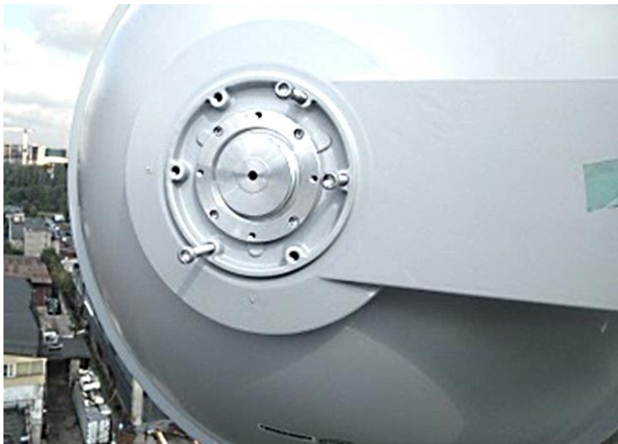
Fig. 41. Install 3 bolts on positions of "5, 15 and 35 minutes" on the antenna flange
