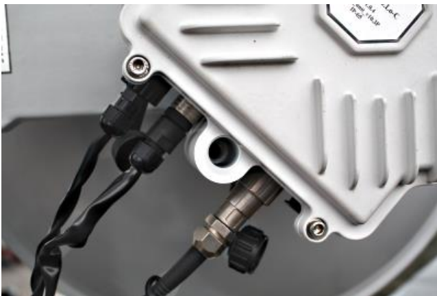
Fig. 21. Position of sockets to be directed down, not up
