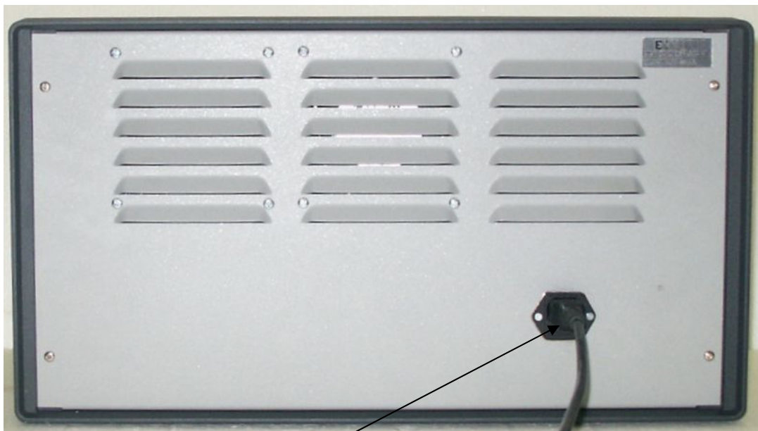
Power plug 220 VAC with built-in fuse 2A
