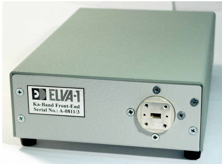
Fig. 7. Ka-band Front-End. Outside view 2.
