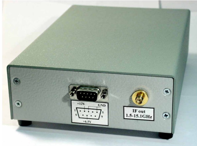
Fig. 6. Ka-band Front-End. Outside view 1.
