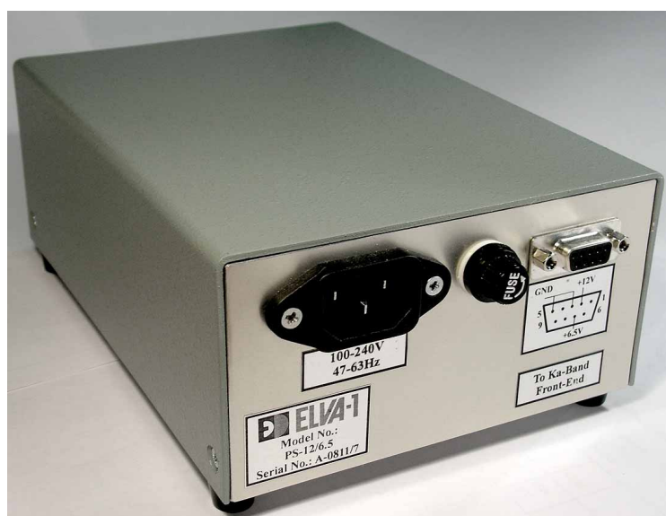
Fig. 12. Power Supply block for Ka-band Front-End. Rear Panel
