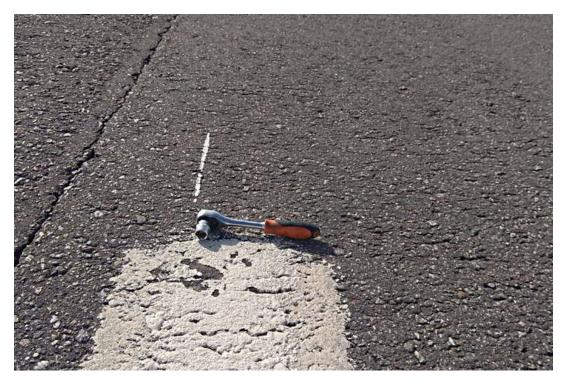
FOD radar successfully detected the entire set of uncalibrated foreign objects. This additionally confirmed the technical characteristics of the equipment and its applicability to detect various FOD targets. Scanning speed of 1.2 miles (2000 m) per minute enables real-time data collection thus expediting identifying FOD sources and facilitating fast runway clearing process.
