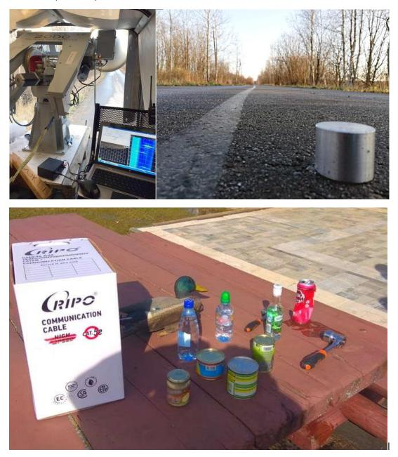
In addition to FAA-recommended reference cylinder Ø3.8 cm and 3.1 cm high, the field experiment was included a demonstration of the detection of a set of 10 different non-calibrated targets scattered on the runway at distances from 0.16 to 0.4 mile (250 m to 650 m), counting from near to radar runway side. These items included two wrenches, water and alcohol bottles, metallic cans, coil with wires, ribbon bird.
