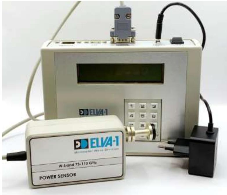
Fig.1. Power meter with the sensor and power supply
