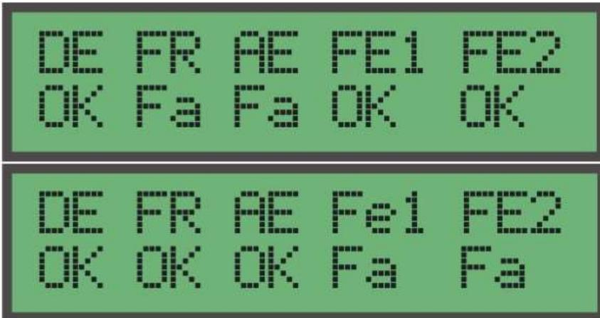
Fig. 11: Failed sensor self-test screens
