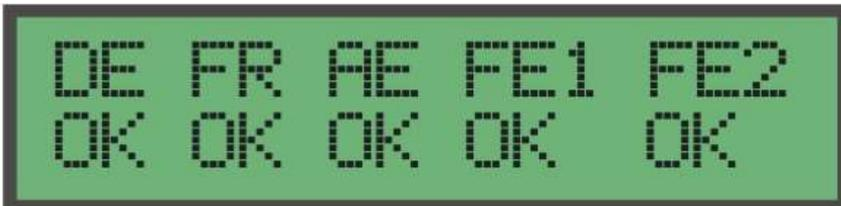
Fig.9. Indication of completed power sensor self-test
