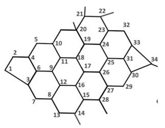
MESH network is a data transmission network consisting of peer nodes that have multiple connections to each other. Traffic is automatically distributed across the nodes of the network by algorithmically finding optimal routes.
