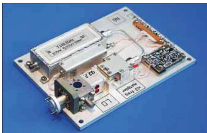
Fig. The 92.2 GHz frequency multiplier and up-converter below are key parts of high stable low phase noise mm-wave source for EPR spectrometer
