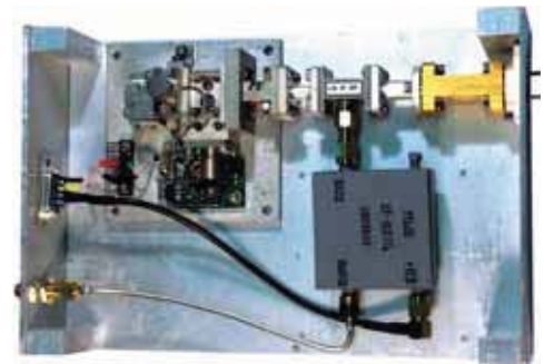
Inside view of E-band front-end of Radiometer for Castor Tokamak
