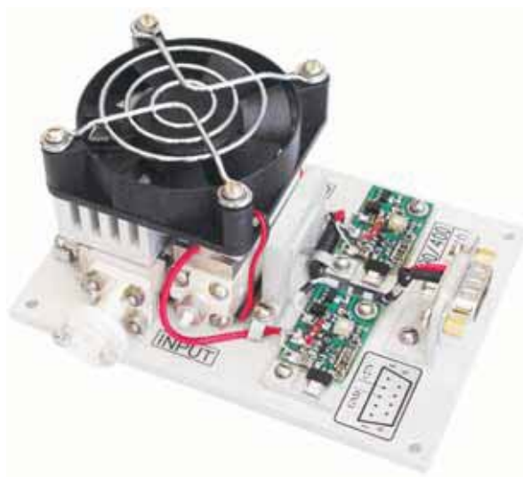
Photo of 400 mW power amplifier produced for special request Input power 160 mW, output power 400 mW, F = 90 GHz
